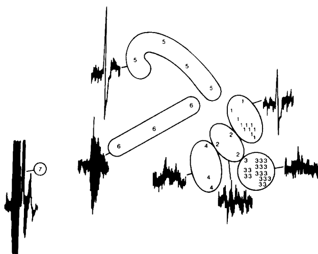
Figure 8 Results of cluster analysis of 64 signals from a sample of propylene + 40% calcium carbonate. (For each cluster the boundaries and a representative signal are indicated)
